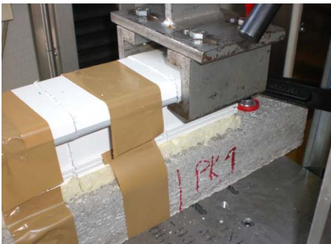
**Fig. 7** Test set-up for tensile test
